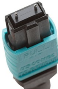
Abbildung 2: Always inspect the individual fibers of the MPO connectors required for high-speed parallel optic applications, since it can be difficult to ensure that all fibers in the array are free of contamination.
